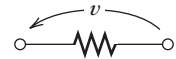
Figure 1.13 The positive reference for v is at the head of the arrow.
